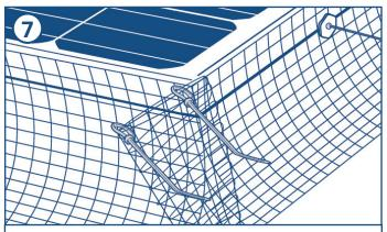
Secure the folded flap against the mesh with a couple of cable ties.
