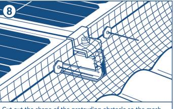
Cut out the shape of the protruding obstacle so the mesh sits flush against the panel without leaving any gaps.
