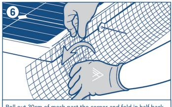
Roll out 30cm of mesh past the corner and fold in half back onto the corner, fold access flap diagonally to secure.
