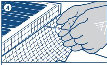
Slide the locking disc onto the rod and push firmly to secure the mesh tightly.
