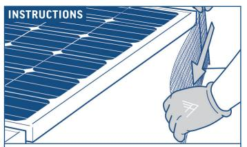
Roll out the mesh and align the top edge of the mesh along the side of the solar panel.
