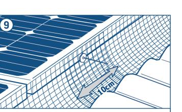
Overlap the start with approximately 10cm mesh to completely wrap the perimeter. Secure with cable ties and insert a fastener through the overlapped pieces and cut away any excess mesh.
