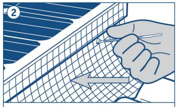
Insert the head of the fastening rod through the first mesh grid below the panel frame.
