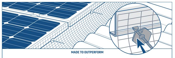
Comprised of premium grade 304 stainless steel mesh, coated across the entire width with UV resistant PVC. This ensures no part of the steel mesh is exposed to potentially scratch the roof and solar panels or to become corrosion points.
